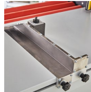
Magnetic feeding guides for quick and accurate substrate alignment
